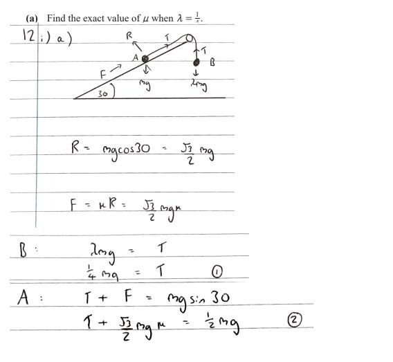
(i) It is given that A is on the point of moving down the plane.
